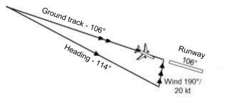
Fig. 7. The wind correction for wind from 190 at 20 kt, and at an airspeed of 139 kt is  $8.5^{\circ}$  to the right.
