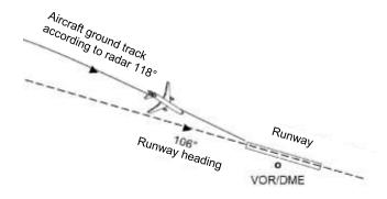
Fig. 5. Wind correction for wind from  $190^{\circ}$  at 20 kt, and at an airspeed of 139 kt is  $8^{\circ}$  to the right. Therefore the heading must have been  $126^{\circ}$  (consistent with the DFDR).
