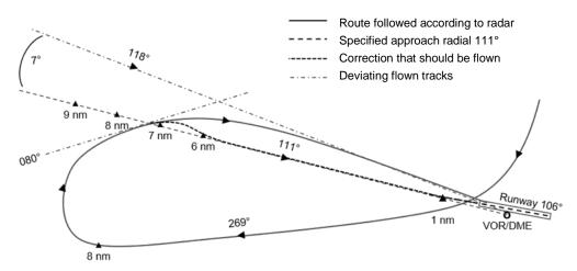
Fig. 4. Approach to Faro airport, based on the Approach Chart in Appendix 2.
